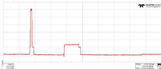
Figure 5: Current measurement of transmitting and receiving 10 bytes
